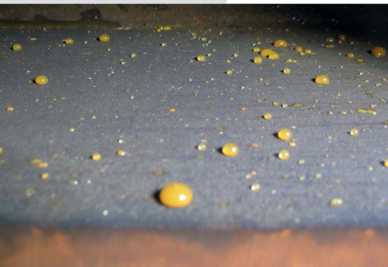
Hydrophobic surfaces in condenser
